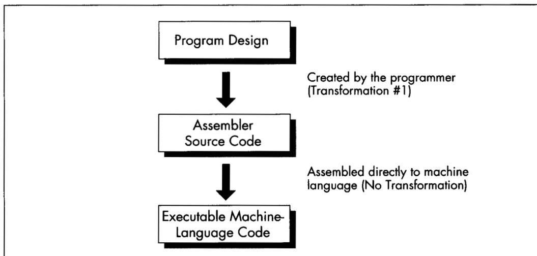
*Properly constructed assembly programs suffer no transformation loss.*
