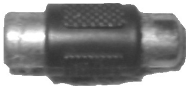
Figure 1.26 You can use an inline connector to hook the Atari up to your TV using a modern RF switch.
