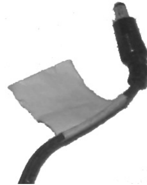
Figure 1.19 This side of the power supply plugs into the Atari's power port.
