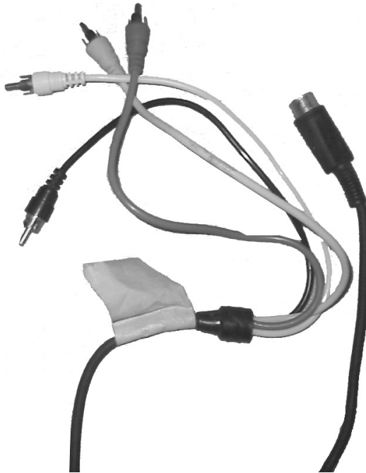
Figure 1.17 Generic Video Cable: This is used to connect the Atari to a computer monitor.
