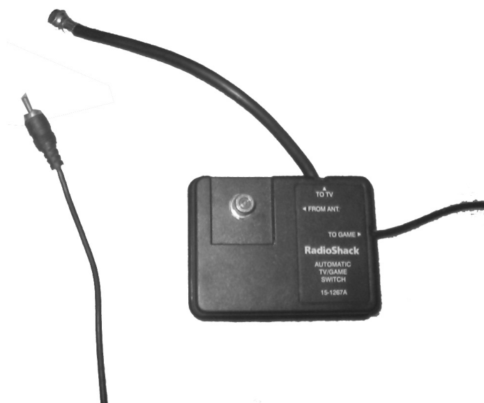
Figure 1.35 If you are using a TV, you need a TV switch box (sometimes called an RF switch).
